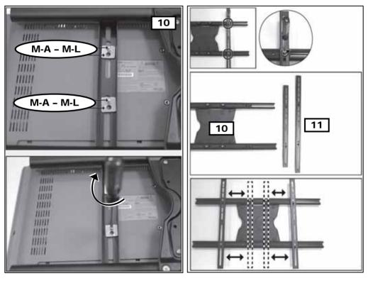
**Note**: IF MONITOR SCREWS "BOTTOM OUT", THEN USE ADDITIONAL WASHERS (not included) TO TAKE UP THE SLACK.
